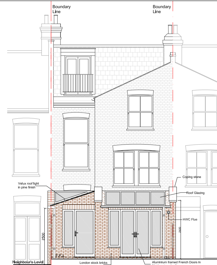
PROPOSED REAR ELEVATION SCALE 1:100
