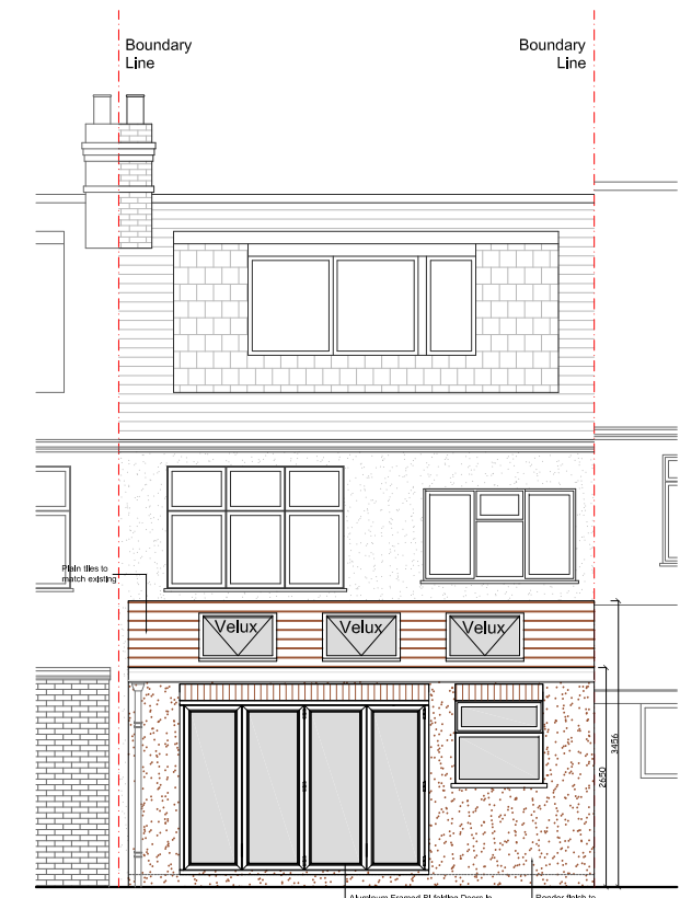
PROPOSED REAR ELEVATION SCALE 1:100
