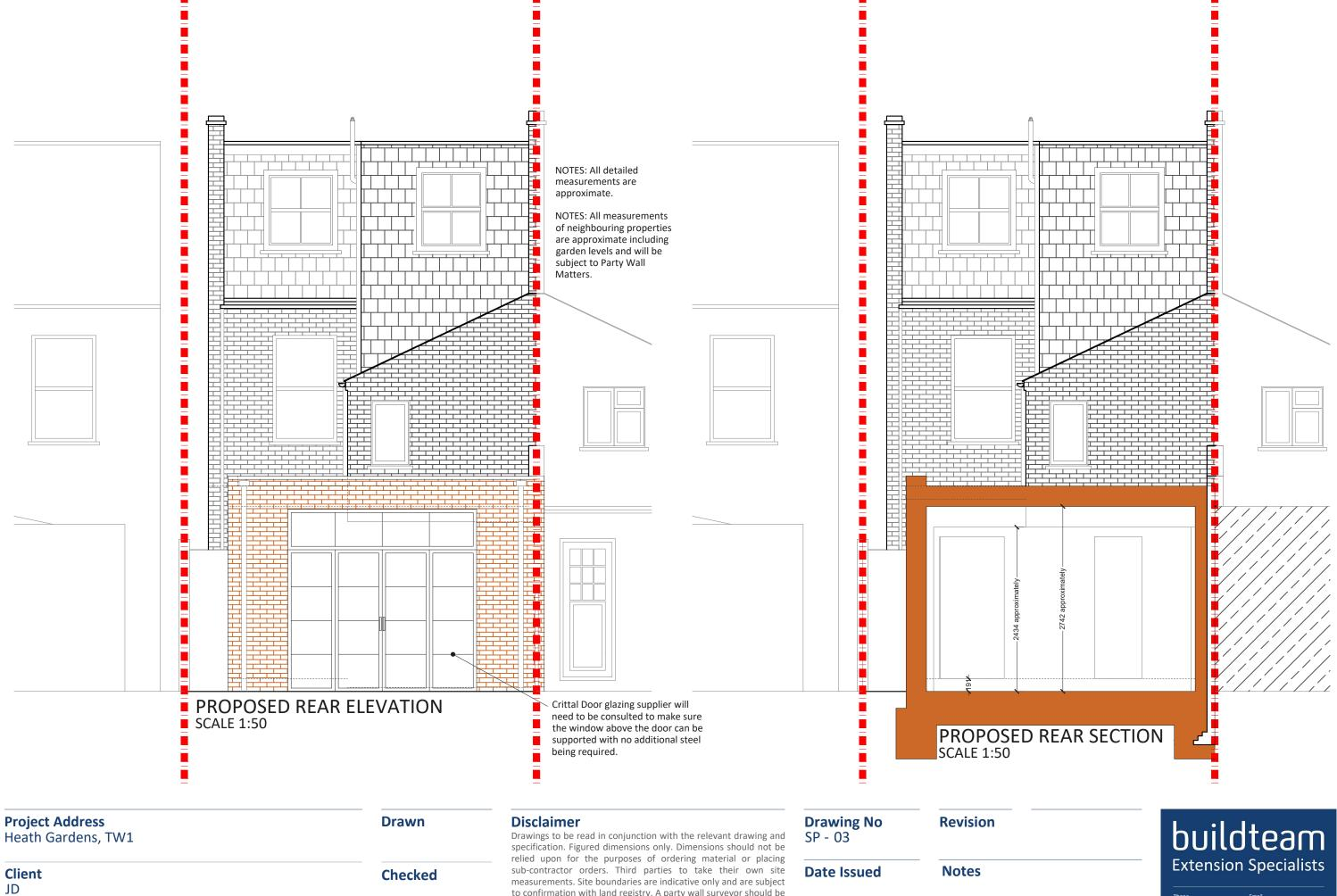
**Drawing Title Proposed Rear Elevation & Section**  to confirmation with land registry. A party wall surveyor should be consulted to ascertain whether adjoining owners are notifiable. On planning drawings, all structural beams, openings, lintels and any other bearings are indicative and are subject to review from a
