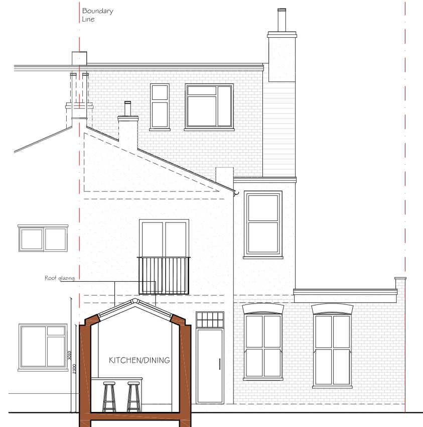
PROPOSED SECTIONAL ELEVATION A-A SCALE 1:100
