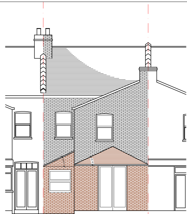
PROPOSED REAR ELEVATION SCALE 1:100
