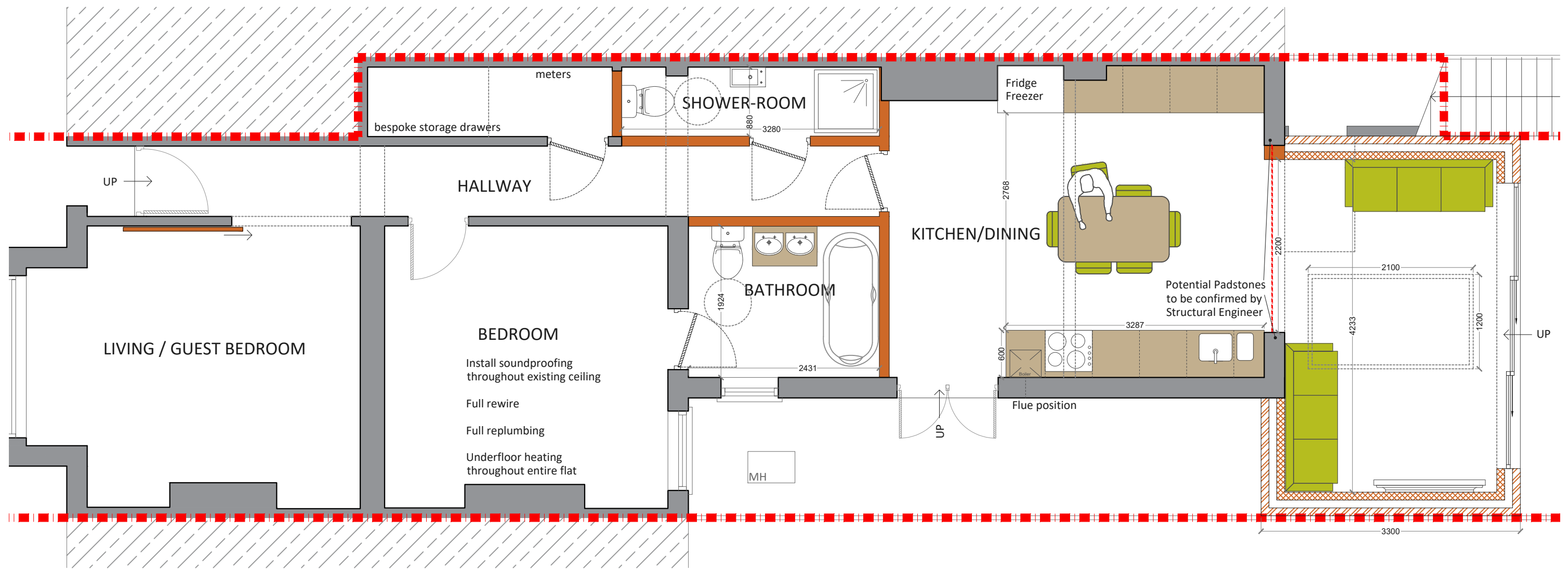
PROPOSED GROUND FLOOR PLAN SCALE 1:50
